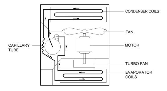
Figure 32 is a brief description of the important components and their function in what is called the refrigeration system. This will help you to understand the refrigeration cycle and the flow of the refrigerant in the cooling cycle.
